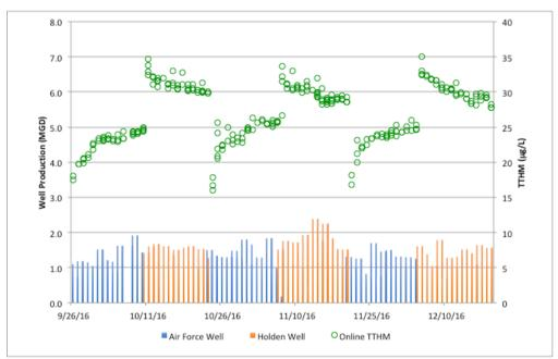
The data clearly depicted that the biweekly well switch had a significant impact on THM levels leaving the facility.
