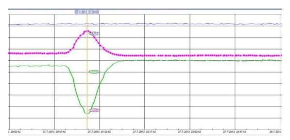
Figure 6-19 Screenshot from Waternet SCADA Interface, Showing a Failure in Ozone Supply (green) and Coinciding Increase in the UV Parameter (blue) Indicating the Change in Absorption due to Ozonation Decrease. ΔUV is Related to the Amount of Organic Material that has Reacted with Ozone, and therefore an Indicator of the Amount of Ozone Dosed. The Failure Was Detected Based on ΔUV Before the Control Room Reported the Issue.
